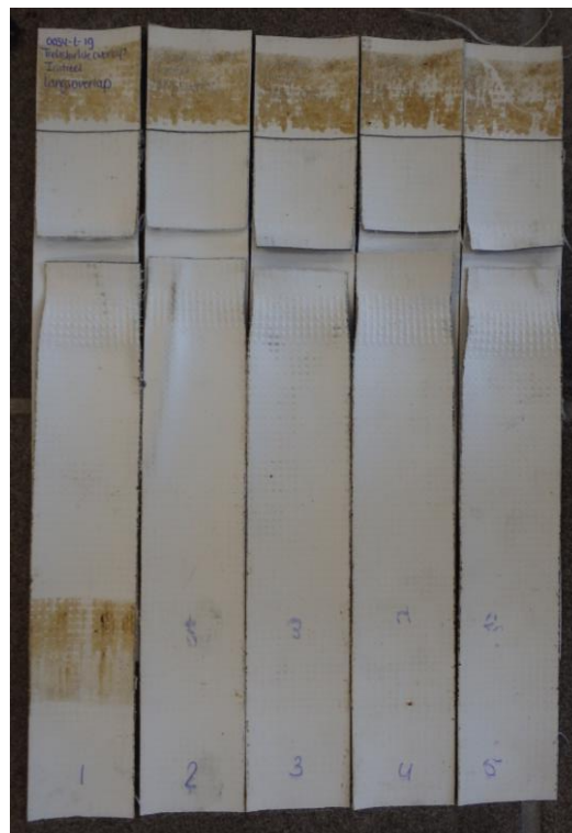
Photo 2 Failure mode seam strength, transverse direction, initial.
