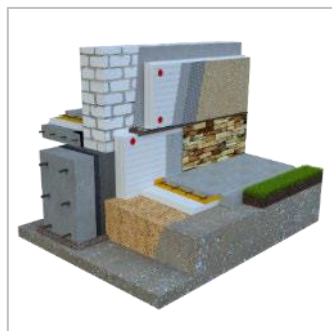
Fastening XPS to waterproofing
