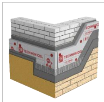
Fastening XPS on basement to decking
