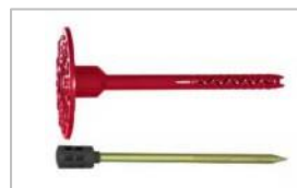
Disk-shaped facade anchor. Consumption 5-7 pcs/m 2
