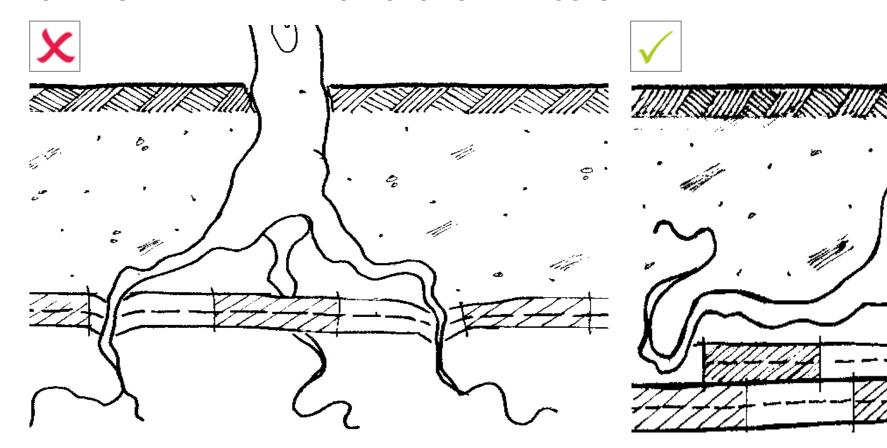
Traditional bitumen membranes are organic, so roots can grow in them, and, over the time, penetrate throughout the bitumen layer and damage the roof and waterproofing system. Bitumen membranes for green roofs contain chemical compound that does not allow roots to penetrate, at the same time it does not have a negative impact on the plant and the environment.
