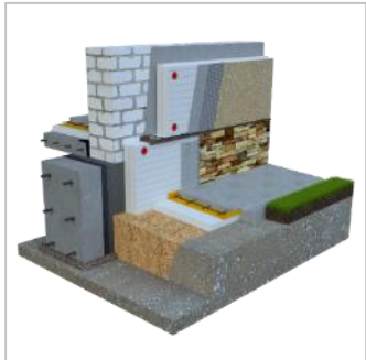
Fastening XPS to waterproofing
