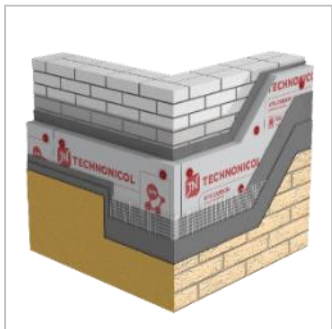
Fastening XPS on basement to decking
