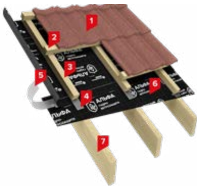
Fig. 5. Structure of the TN SCMRT Classic roofing system
