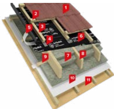
Fig. 6. Structure of the TN SCMRT Attic roofing system
