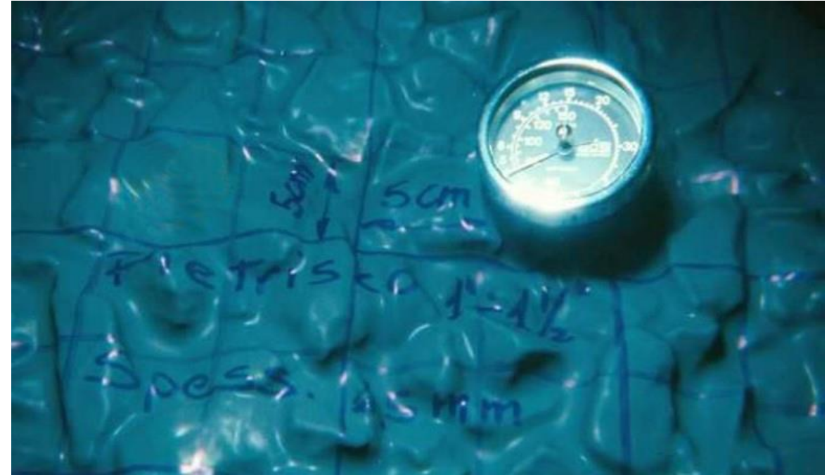
Unreinforced PVC-P membrane at a depth of 50 m.
