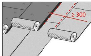
Cap sheet membrane should be positioned at a distance of min. 300 mm from overlaps of underlay to the water flow.
