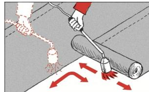
Heat the material and the base on all width of the roll, overlaps must be heated additionally.
