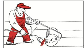
Heat the base and the bottom side of material at the same time to get a small bitumen flow.
