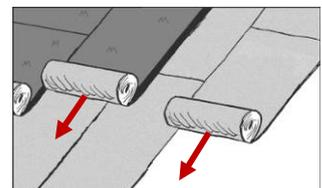
**NOTE:** Cap sheet membrane is installed in the same way as underlay membrane. It is forbidden to install roll materials in a crossway.
