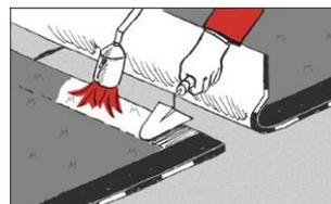
In places of end overlaps of the cap sheet membrane the top side of the material (with slate) must be additionally heated by torch. Then the slate is pressed into bitumen by spatula to increase the adhesion of the following roll.
