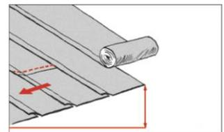
On roofs with a slope <15% membranes are rolled out perpendicularly along the water flow.
