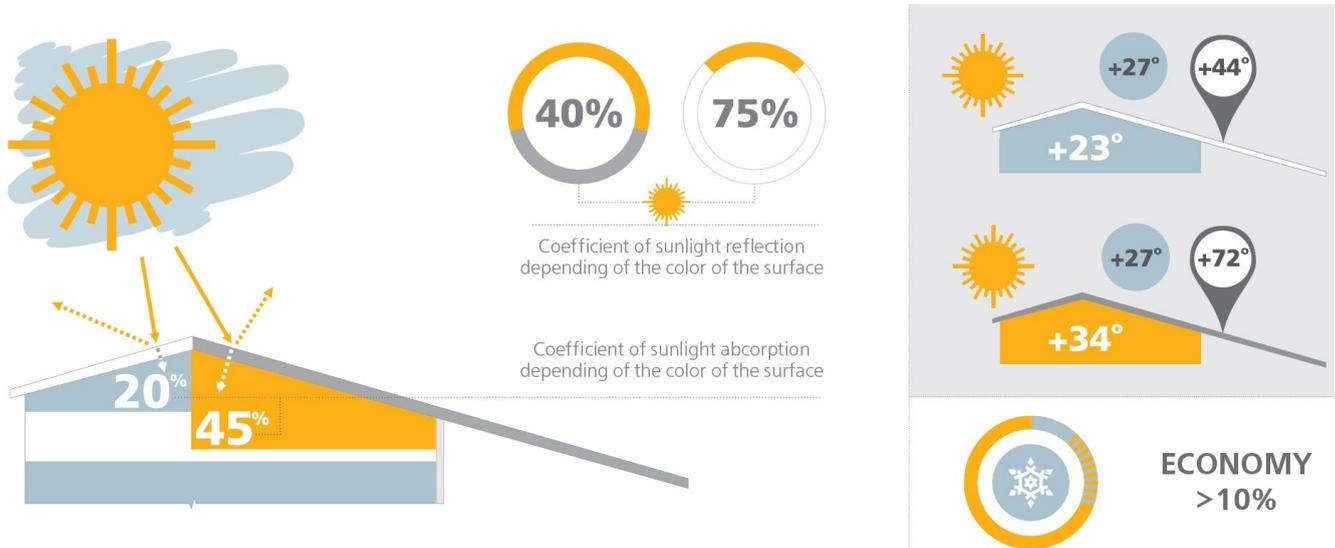
Using of TECHNOMICOL ENVIRO WHITE roofing membrane with a high solar reflective index allows reducing the quantity of heat from the sun getting to the inside of the house from 45% to 20%, thereby reducing the costs of conditioning the premises under the roof (on sunny days) by 10-30%. Your roof stays cool.
