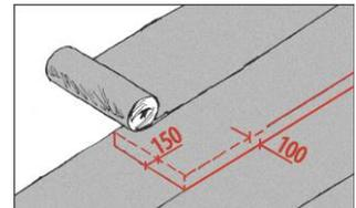
Longitudinal overlaps should be 100 mm; end overlaps should be not less than 150 mm.
